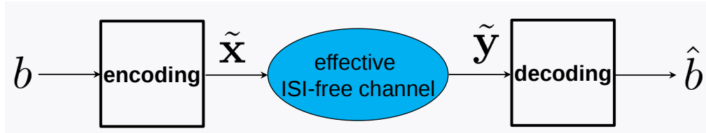
Figure 2: How to map information bits into frequency-domain signals in OFDM.
