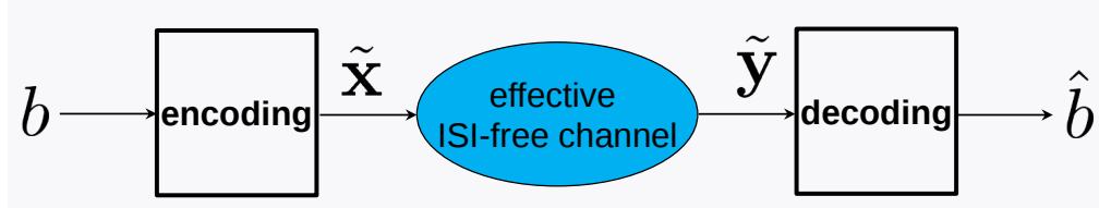
Figure 4: How to map information bits into frequency-domain signals in OFDM.
