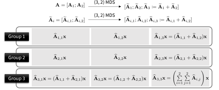
Fig. 3. Allocation of the computational task to workers in a (3, 2) \times (3, 2) coded computation
