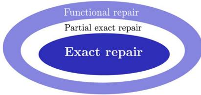
Fig. 3. Repair models for distributed storage systems. In exact-repair, the failed nodes are exactly regenerated, thus restoring lost encoded fragments with their exact replicas. In functional-repair, the requirement is relaxed: the newly generated node can contain different data from that of the failed node as long as the repaired system maintains the MDS-code property. In partial exact-repair, only systematic nodes are repaired exactly, while parity nodes are repaired only functionally.
