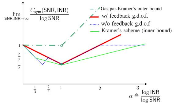
Fig. 4. The generalized degrees-of-freedom of the optimum and Kramer's scheme
