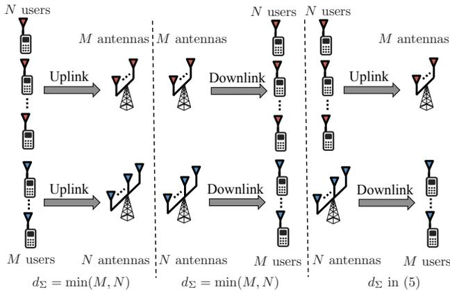
Fig. 3. Sum DoF for uplink, downlink, and uplink-downlink operation for  $M_1 = N_2 = M$  and  $M_2 = N_1 = N$ .
