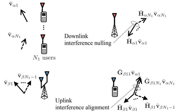
Fig. 4.  $d_\Sigma$ -achievable transmit beamforming for  $M_2 = 2$ ,  $M_1 = N_2 = 1$ .
